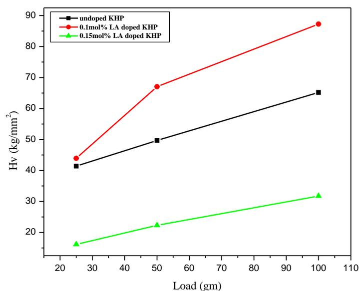
Fig 5: Vickers hardness vs load of Undoped and LA doped KHP crystals
